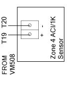
nstalling the ACI/1K-2W-RH3-R Temperature and Humidity Sensor and the ACI/1K-2W-R Temperature Sensor
